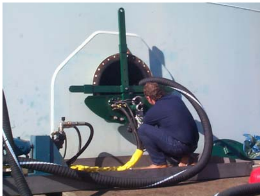
Fitting Cannon in manway
